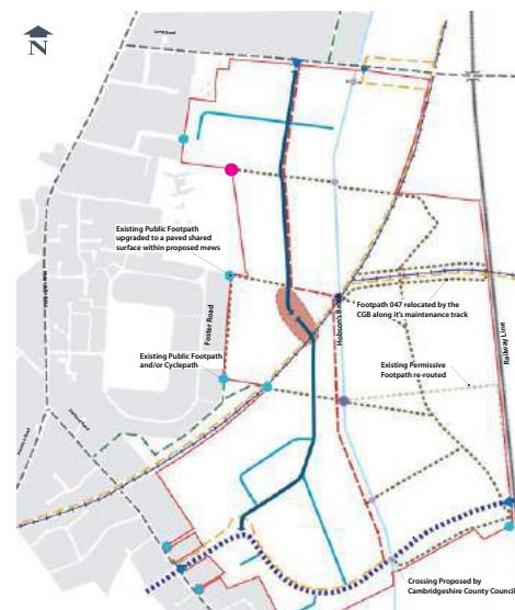
Fig. 104: PP2 Movement and Access Parameter Plan Note 1: The alignment of the paths in the Green Corridor are indicative only and the details will be determined through approval of the comprehensive landscape plan Note 2: The exact alignment of the proposed routes will be subject to the final design Note 3: Parameter Plan (PP2) revised in April 2010
