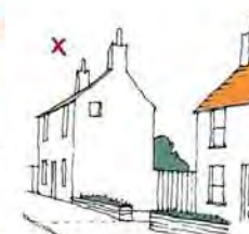
Low walls, hedges or fences appear minuscule in scale and fail to offer any sense of 'protection' to the pedestrian
