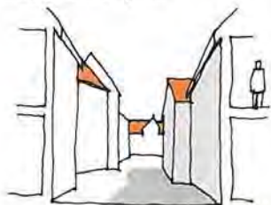
Width of space equal to or less than height of enclosing planes
