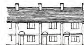
Front elevation with larger openings and facade subdivided to emphasise individual houses
