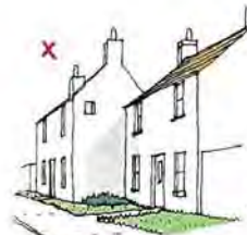
Indeterminate grassed or planted area in front visually detaches building from street to detriment of townscape
